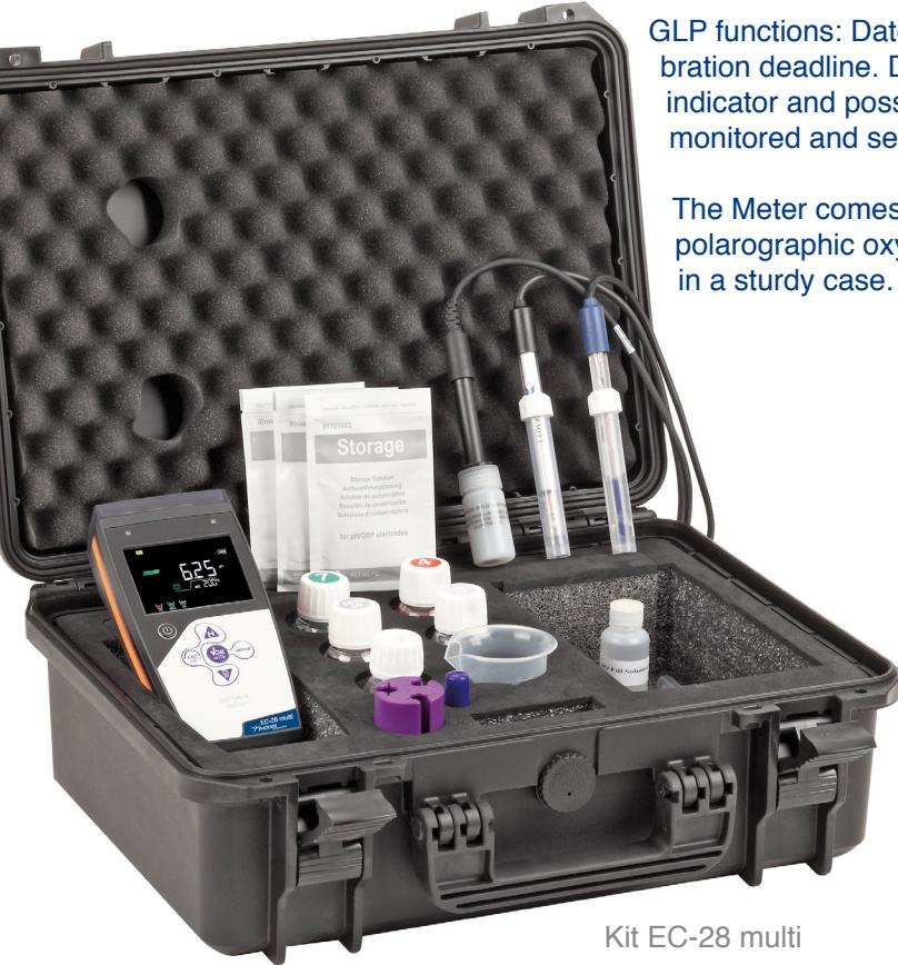
GLP functions: Date and time, display of calibration data and setting of calibration deadline. Data logger with download possibility. Measurement stability indicator and possibility to select 3 stability levels. All operations are constantly monitored and self-diagnosis messages.
